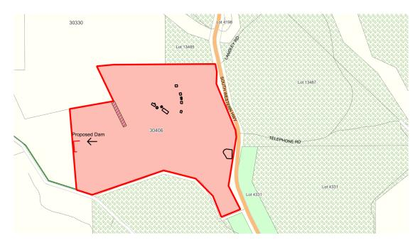
Plans and details submitted with the application indicate that the dam wall, adjacent to the neighbouring property boundary is 50 metres in length and projects back into the property for 80 metres. The internal depth of the dam is 5 metres and a wall height of 2 metres. The dam will have a total capacity of 80
