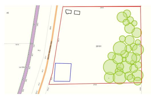
Plans and details submitted with the application indicate that the dam is to be setback 5m from the southern and western boundary. The dam wall, adjacent to the neighbouring property boundary is 50 metres in length and projects back
