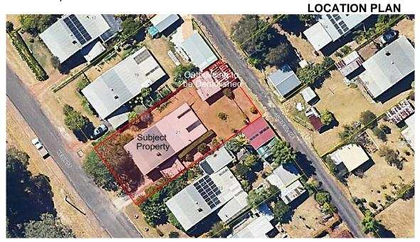
The application is proposing the demolition of the existing Outbuilding which is located at the rear of the property and the replacement with a 9m by 6m (54m²) Colorbond® Outbuilding. The proposed Outbuilding is to be constructed with a 0.05m setback to the rear and 0.09m to the side boundary and is to be constructed of steel, in the Colorbond® colours of Wallaby and Windspray.
