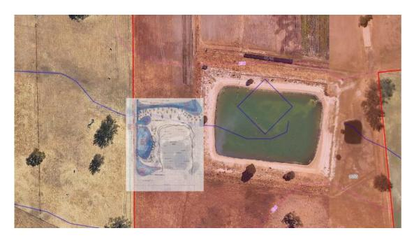
The applicant is seeking retrospective planning approval for drainage works carried out along the western boundary of their subject property including the construction of a series of drains and ponds to direct and slow down the flow of the water on the subject property. These works are in conjunction with proposed works to recontour the property to improve their arable land for intensive agricultural purposes.
