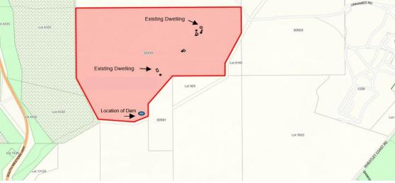
The applicant is seeking retrospective planning approval for a 29m long and 45m wide dam. The applicants excavated an existing 2.9m round soak and utilised the slope of the land to form the dam walls. The plans indicate a 3m wide wall with the toe of the dam wall 8m to the boundary. As part of the approval, the applicant is also proposing to expand the dam capacity by moving the dam walls, 5m to the east and north and 10m to the west.
