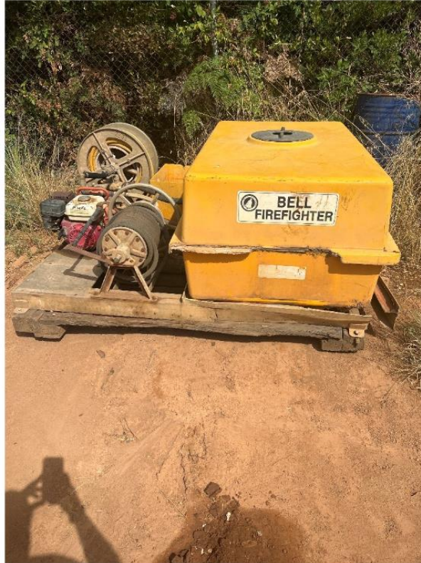
Un-repairable slip-on unit
