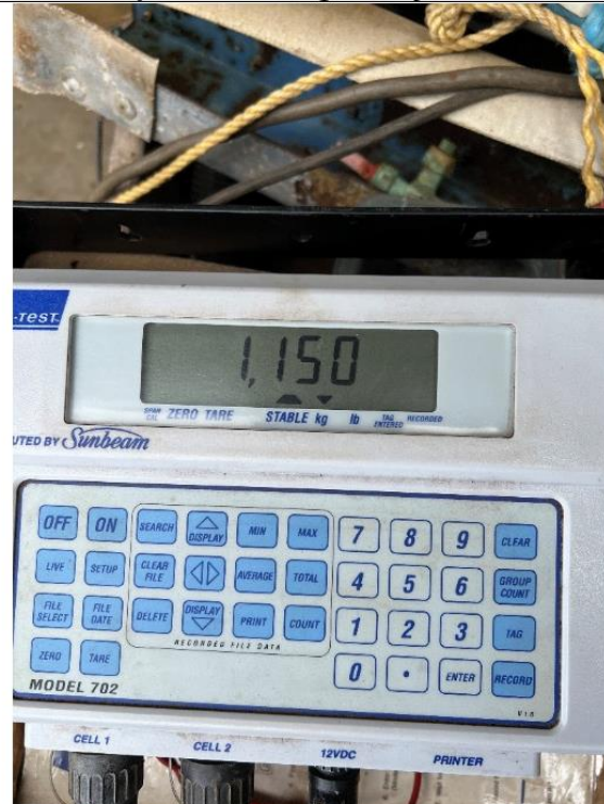
Slip-on unit weight fully loaded
