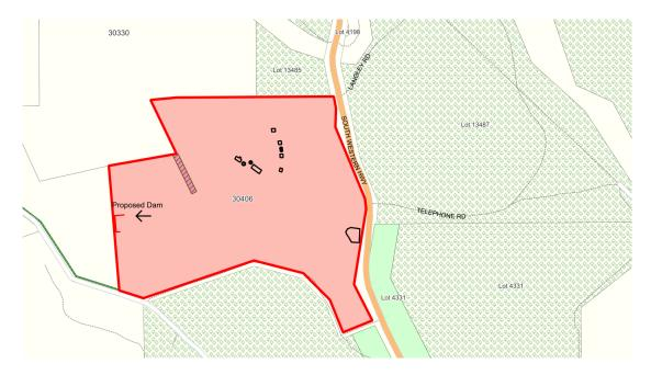
Plans and details submitted with the application indicate that the dam wall, adjacent to the neighbouring property boundary is 50 metres in length and projects back into the property for 80 metres. The internal depth of the dam is 5 metres and a wall height of 2 metres. The dam will have a total capacity of 80 mega litres. The proposed dam is intended to be used for stock water. A
